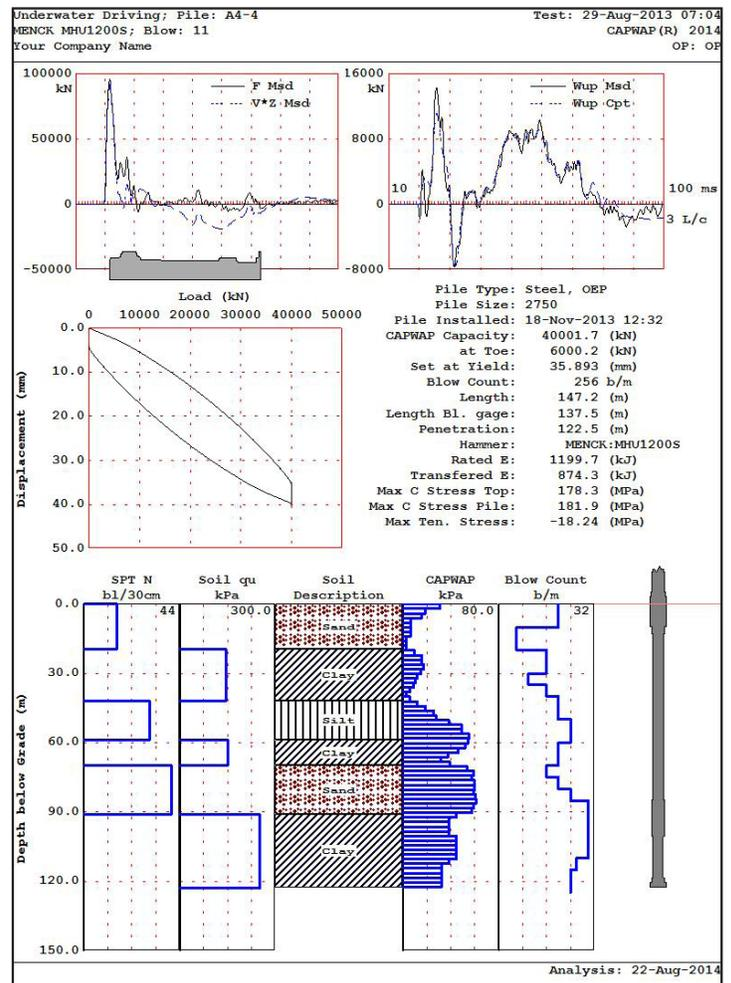
**Pile Dynamics, Inc. (PDI)** is the world leader in developing, manufacturing and supplying state of the art QA/QC products and systems for the deep foundations industry. The company is headquartered in Cleveland, Ohio, USA, with offices and representatives worldwide. For additional information visit us at [www.pile.com](http://www.pile.com) or contact [info@pile.com](mailto:info@pile.com).
