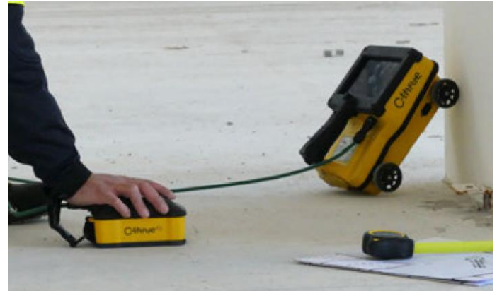
C-thrue XS can be connected via LAN to the C-thrue device allowing for a real-time visualization of the collected data on the multi-touch display.
