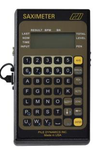
confirm assumptions made when analyzing the pile by the Wave Equation (GRLWEAP Software Program). For hammers other than Open End Diesel, optional accessories allow computation of kinetic energy.
